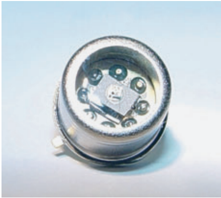
Figure 3: Si-APD in a standard TO5 package (diameter 8 mm), suitable for wavelengths from 350 nm up to 900 nm
