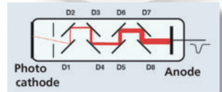
Figure 1: Schematic illustrating the principle of a conventional photomultiplier tube (PMT) (image courtesy of Becker&Hickl)
