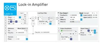
Every demodulator has a graphical representation in the form of a block-diagram for intuitive instrument control. In addition, the overview tab allows the control of all demodulators, signal inputs and signal outputs from a single panel.
