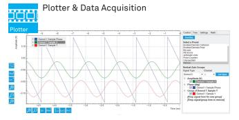
The Plotter and Data Acquisition module display multiple measurement data in the time domain. The Plotter displays the data continuously and the Data Acquisition module captures and displays individual shots based on numerous internal and external trigger conditions.
