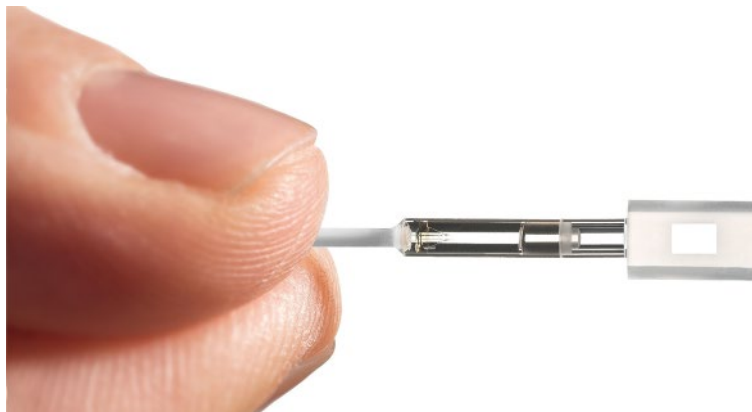
Fig. 1 Sensor head connected to an optical fiber: centerpiece of the optical microphone is the miniature Fabry-Pérot etalon shown on the right side of the picture. Sound enters the etalon through the air gap between the mirror surfaces. Small size and robust dimensioning of the glass elements prevent the influence of mechanical vibrations to be below the sensor self-noise throughout the full measurement range.
