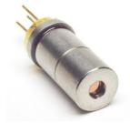
NECSEL presents a VBG® wavelength stabilized 785.0nm laser diode in a compact TO-56 can based coaxial package. The NECSEL patented VBG® wavelength stabilization method offers a stable operation over a wide range of operational temperatures and power levels. The compact, low cost TO package makes this product applicable to many uses. An internal  $10k\Omega$  Thermistor allows for accurate temperature monitoring of laser diode to facilitate
