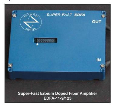
This EDFA is designed to be used in the traditional C-band. During operation, the signal wavelengths must be confined to a 3.2 nm region for each optical amplifier, although the band may be anywhere within the C-band. The unit can work with up to 4 channels.
