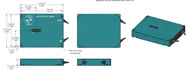
Figure 1. Super-Fast Optical Amplifier Mechanical Specification
