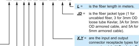
connector receptacle types for connector style U-Brackets. For pigtail style U-Brackets they refer to the male connectors on the fiber ends (3 for NTT-FC, 5 for SMA 905, 8 for AT&T-ST, SC for SC connectors, X for unterminated fibers, etc.).
