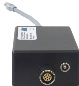
Figure 4: Cable box for signal processing outside vacuum
