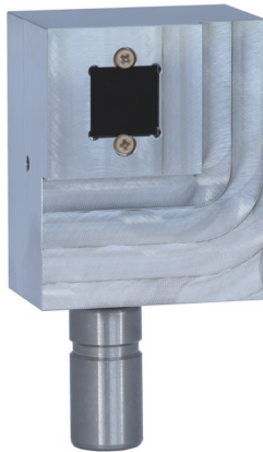
Figure 2: Front side of clean room and vacuum detector
