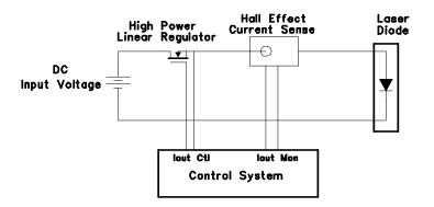
Figure 2 Simplified LDQCW Block Diagram
