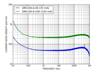
The DRV100 laser driver <u>current noise was measured</u> across a 30  $\Omega$  resistor for the 40 mA laser current version (A-40) and a 5  $\Omega$  resistor for the 200 mA laser current version (A-200).
