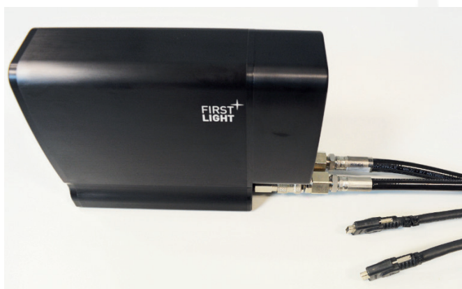
Figure 6 : CameraLink SDR-26 connector and cable
