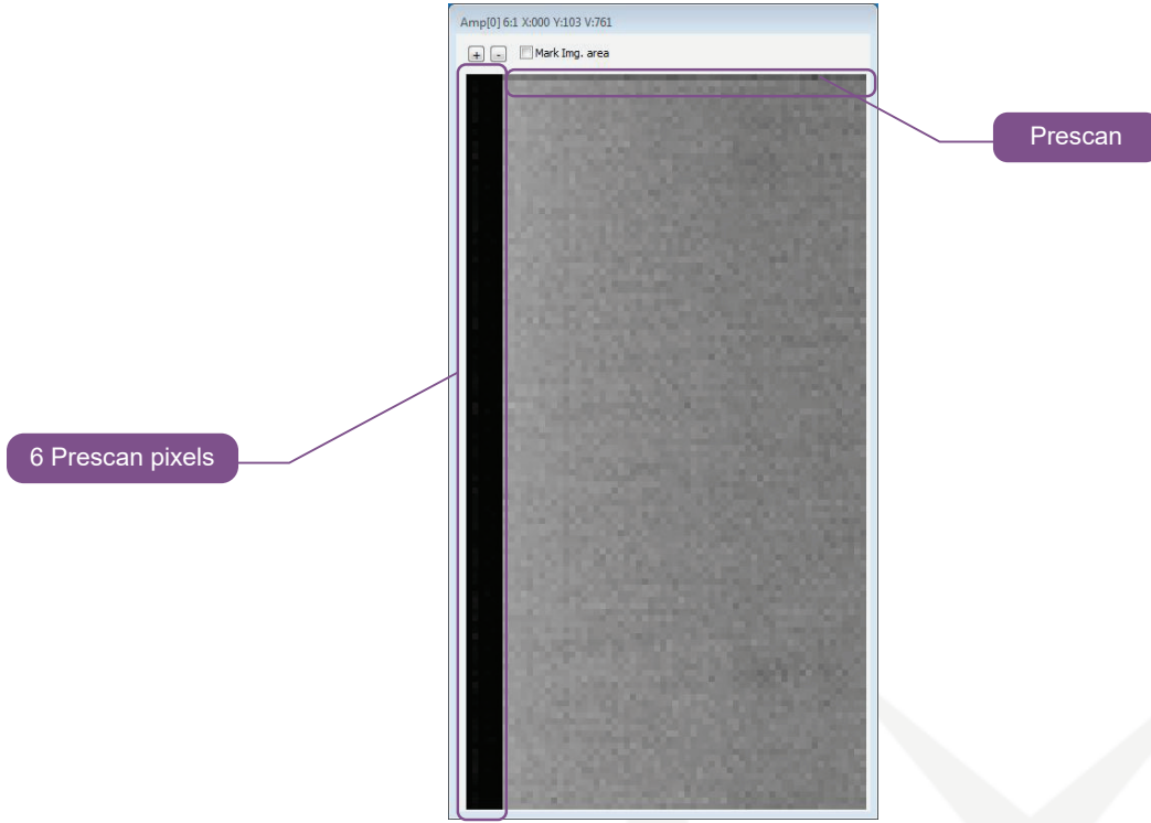
Figure 16 : Single Amplifier image showing prescan data
