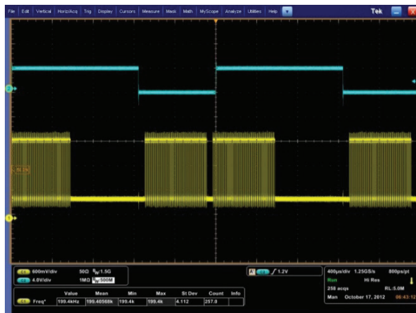
Figure 26 : Double frame triggered with long synchro in signal
