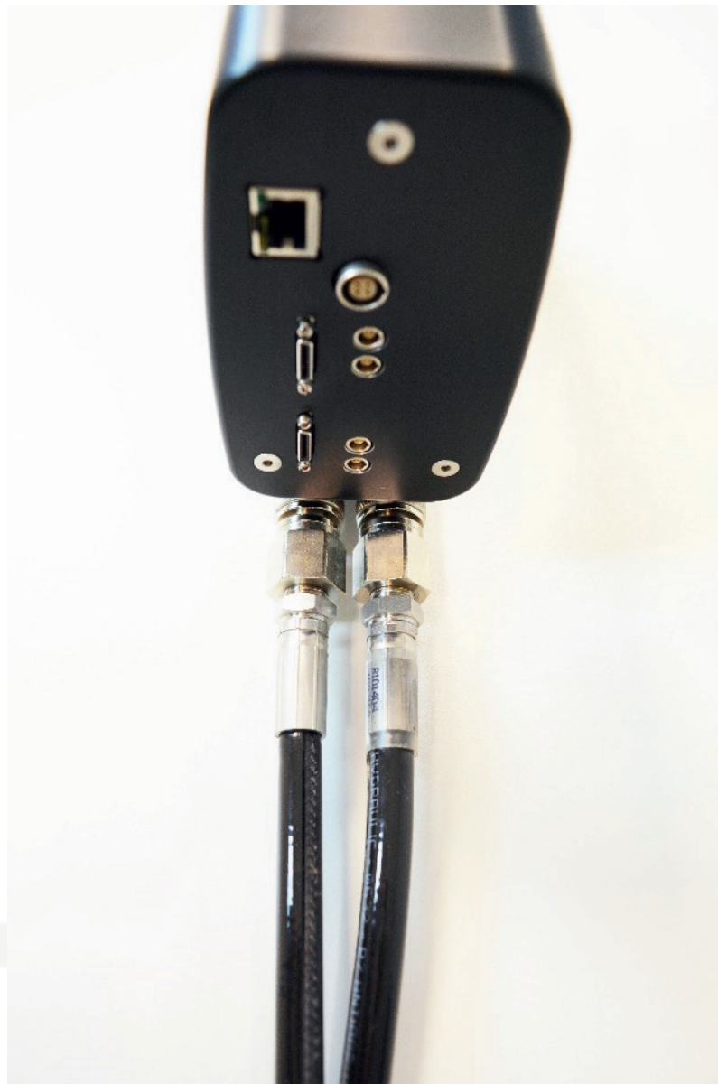
Figure 5 : Coolant connectors in place
