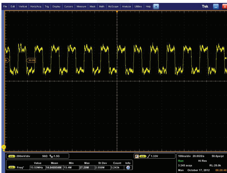
Figure 30 : Pixel clock signal at 18.64 MHz
