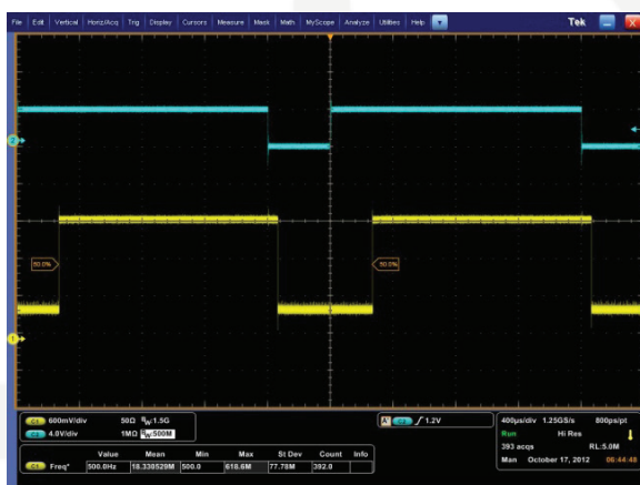
Figure 22 : Input and output signal display. Input is blue, output is yellow
