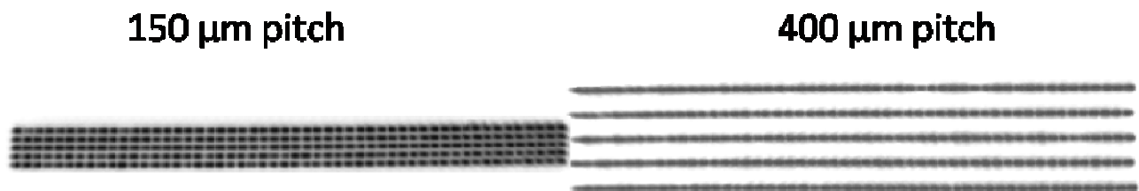
Figure 5. Comparison of example near-field images from a High Density Stack (left) and a standard array with 400 \mu\text{m} pitch (right). Each array contains five bars.
