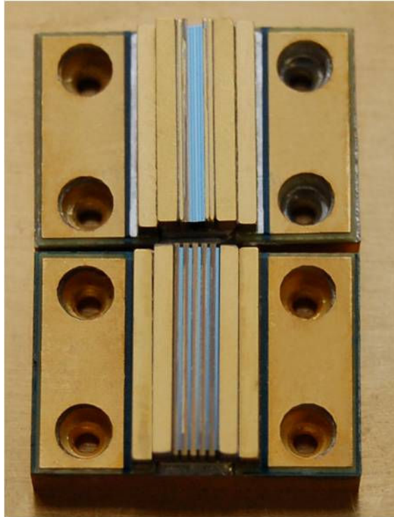
Figure 4. Photograph of two 5-bar stacks placed end-to-end. The High Density Stack is on the top and a standard array with 400 \mu\text{m} pitch is on the bottom.
