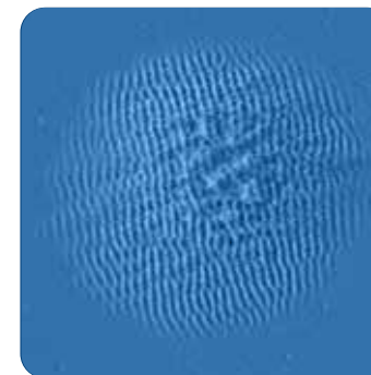
Surface functionalization with conventional system (Gaussian Beam)
