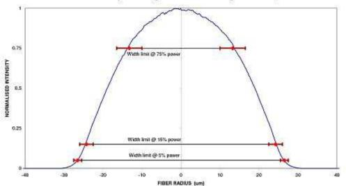
Near Field Intensity Plot showing 65% limits measured using MPX Modal Explorer
