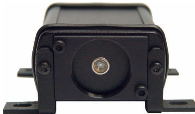
Figure 2. Single photon detector module: id100
