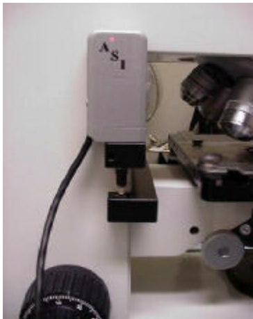
Figure 1. The optional Z-Axis linear encoder monitors the position of the stage.
