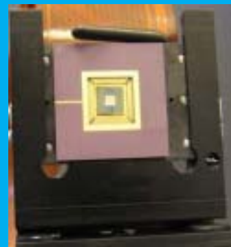
The BMC \mu DM System consists of a 140 channel HV Driver, PC controller, \mu Drive™ software, mirror mount and \mu DM.
