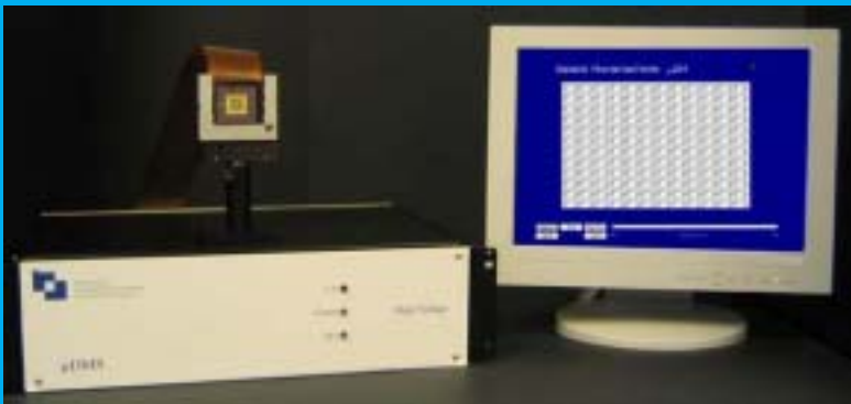
The BMC \mu DM System consists of a 140 channel HV Driver, PC controller, \mu Drive™ software, mirror mount and \mu DM.
