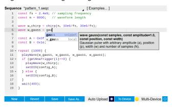
The LabOne UI is designed to get you going quickly by providing hardware control in an intuitive and easily readable form. After defining the waveforms and sequences in the LabOne AWG Sequencer, the LabOne AWG Compiler translates it into machine language and transfers it to the hardware in a minimum amount of time. LabOne sequencing supports loops with dynamically varying delay and conditional branching points.
