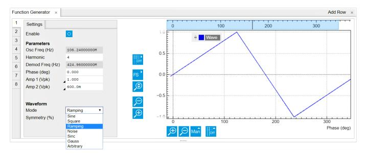
The Function Generator tab in the LabOne UI gives direct access to standard waveform definitions and displays a preview according to the set parameters. These standard signal shapes with tunable frequencies can be multiplied with or added to the AWG waveforms.
