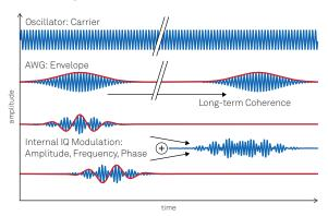
The HDAWG is equipped with digital oscillators to generate the sinusoidal carrier of a signal independently of the programmed AWG envelope signal. This means that long signals can be generated with very fast waveform upload and precise phase coherence across many pulses. Carrier frequencies and phases that would otherwise be written to a static waveform can be freely adjusted and swept.
