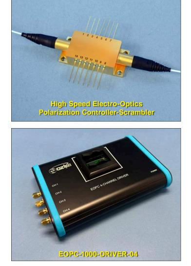
motionless and vibration free design allows fast linear response with less than 10 µs response time to the control signal. The controller's rapid response speed easily handles changes in polarization, caused by the external environment, and is highly suitable for polarization controlling and scrambling to either average PDL and PDG effects, or for making PMD, PDL or DOP measurements. This makes it ideal for precise test and measurement applications.
