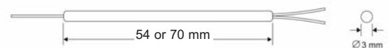
Figure 1: Dimensions of 1x2 or 2x2 Fused Splitter with 250 Micron or 900 Micron Jacketed Fibers
