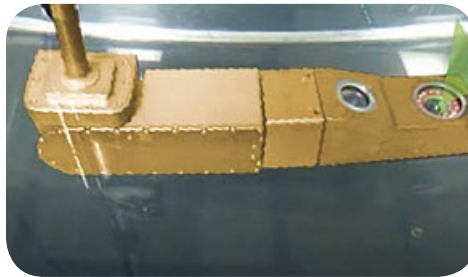
The flexible PT200UW features an operation range of 185 degrees at the "elbow" and infinite rotation at the "wrist."
