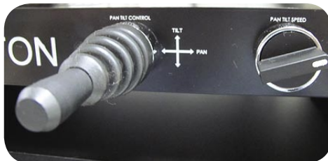
Control consoles for the Newton underwater scanners are fitted with directional and speed controls for the Pan-Tilt Arm on the front panel.
