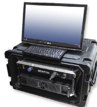
NM200UW Control Console, screen and keyboard with trackball.
