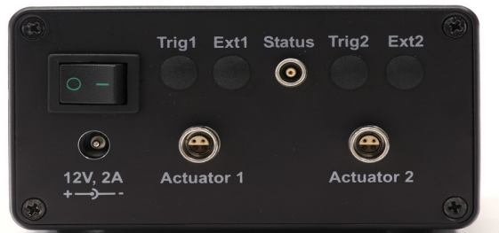
Figure 1: On/off-switch, power plug, and output connections on the left side
