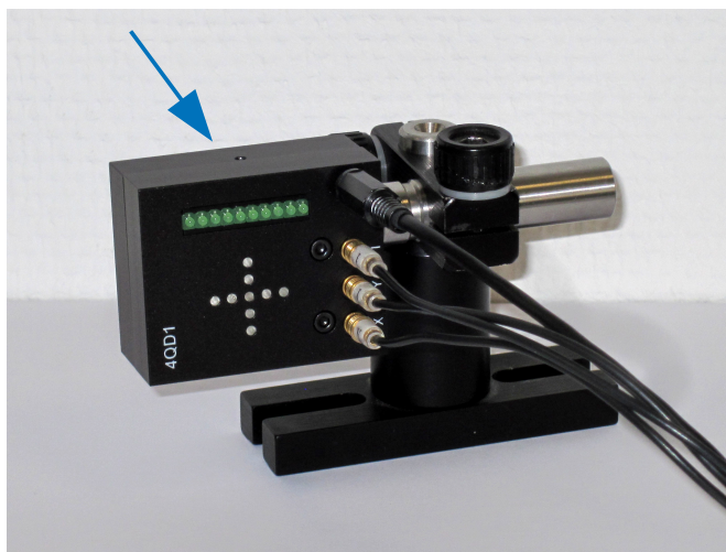
Figure 4: 4-quadrant-diode. The arrow points to the potentiometer for intensity variation (Please use a screwdriver)
