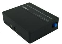
Wavelength and amplitude stability is often a critical requirement for many spectrometer applications. All optical components in the HRS series spectrometers are mounted directly on a single-piece base without using screws. A box enclosure structure further increases stiffness of the base. The proprietary mounting method ensures high stability over time and temperature.
