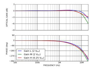
The AC modulation input can be used to modulate the laser above 1 MHz with a modulation gain of 20 mA/V:
