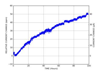
The current stability of the controller after 100 hours is shown below:
