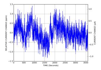
After a subsequent power-on, the CTL101 controller takes only one minute to settle the laser current within 10 ppm of the setpoint value:
