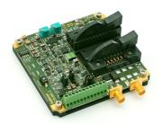
Koheron CTL101 is a low noise current driver with modulation combined with a temperature controller. It is designed to drive narrow-linewidth laser diodes in butterfly package. The CTL101 fits in a 75 mm x 75 mm square, uses a single 5 V supply, and can operate between 0 and 50°C. The CTL101 is conduction-cooled. It comes with an aluminum base plate and a zero insertion force socket for easy mounting.
