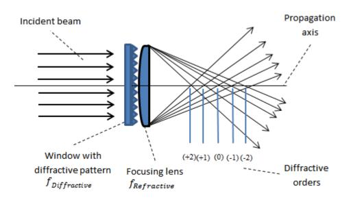
Calculation of the multifocal spots location can be deduced by using Holo/Or's optical calculator (section Multifocal)
