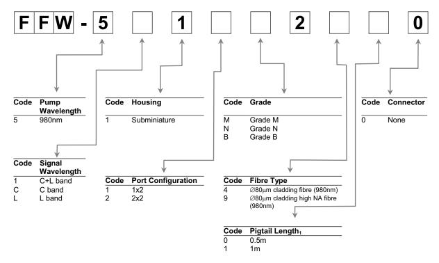
1. Minimum pigtail length. Further pigtail lengths available on request.
