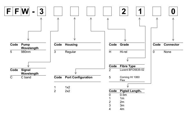
Minimum pigtail length. Further pigtail lengths available on request.
