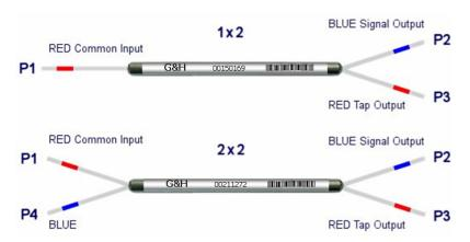
1. 1x2 couplers for blue wavelengths i.e. <500nm are supplied as a 2x2 with an external termination on port P4.
