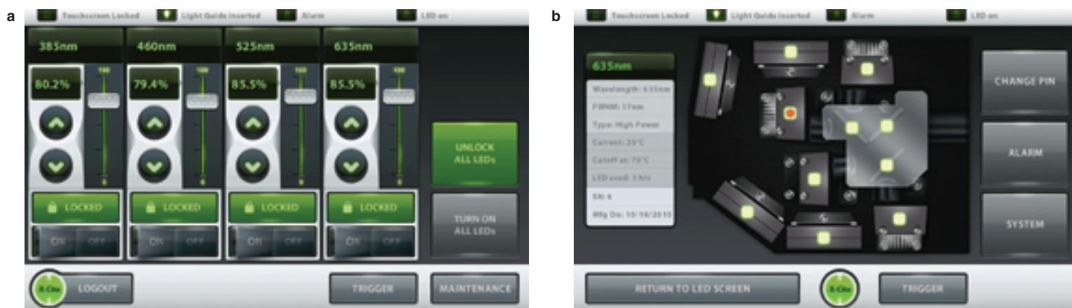
Figure 2 The X-Cite XLED1 features a 7-in. touchscreen display and intuitive user interface.
