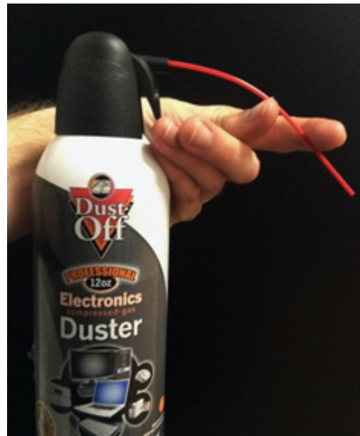
Fig. G.5: Correct vertical orientation of air-duster bottle. Air is blown at an angle by bending the attached plastic nozzle.
