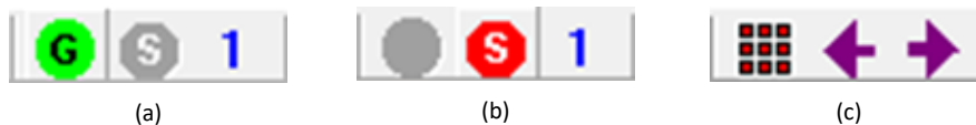
Fig. 2.3: Menu buttons for capturing a live stream or a single image. (a) The green button is used to start capture, while the “1” captures a single image. (b) The red button is used to stop capture. (c) The array button is used to show the images all the images in the Live Stream buffer, whereas the two arrows allow Live Stream buffer image access one image at a time.
