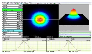
1550 nm beam at 1.268 ms exposure
