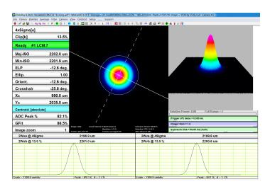
The WinCamD-LCM is paired with DataRay's full-featured software which has no license fees, unlimited installations, and free software updates. It is perfect for applications including: CW and pulsed laser profiling; field servicing of laser systems; optical assembly; instrument alignment; beam wander and logging; R&D; OEM integration; quality control; and M² measurement with available M2DU stages.
