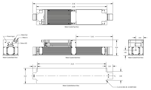
➢ INTEGRATED COOLING/CLASS 4 CONFIGURATIONS (CLASS IV AIR-COOLED SHOWN BELOW)
