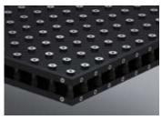
Boards of CA-series are entirely made from carbon fibers. Top and bottom shell consist of several mm thick CFRP shells, structurally joined by tubes made from CFRP. In addition to the advantages of AD-series, boards of CA-series allow the integration of optical/electronical components inside the stiff carbon shell and to route easily wires and optical fibers. Side walls can be installed removeable. Areal weight approx. 19 kg/m².
