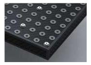
Enhanced version of EC-series. At each mount location a CFRP tube links the top and bottom shell. The CFRP tubes allow easy cleaning of the board, to install removeable additional mounts at the bottom side and to tune the natural frequencies and vibrational damping by inserting adaptive elements. Areal weight approx. 15 kg/m².
