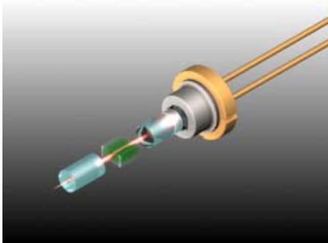
Figure 2. A wavelength-stabilized TO-packaged high-power laser diode with a cylindrical lens and a LuxxMaster™ element installed in front of it.
