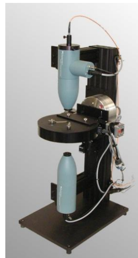
The AxoScan OPMF-1 fixture tilts the sample +/- 55°, with rotation to any angle (0° to 360°)
