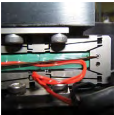
Clamp height motorization with piezo actuator
