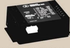
AMI's simmer supplies are powered from a 24VDC source and provide both a built-in automatic ignition restrike circuit and a post-flash boost mechanism. These features minimize the possibility of missing pulses when operating with a continuous train of laser pulses.
